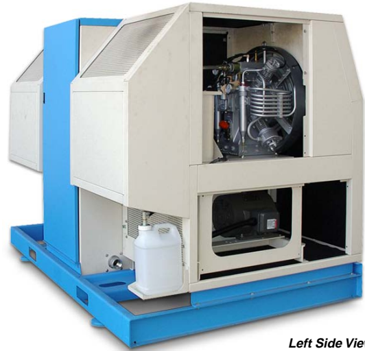
Left Side View: Booster Compressor Module Shown with Access Panels Removed
