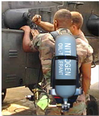
High Pressure Nitrogen Man Portable to "Point of Need" - 4500 psig Lightweight Backpack Cylinder - Part Number: 410780 and Harness - Part Number: 410735-1
